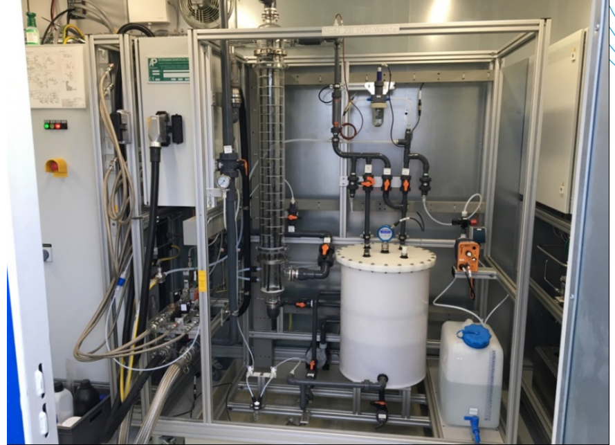
Glass column for technical scale tests
