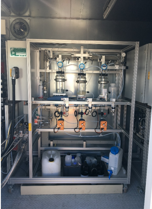
Stirred glass reactors for lab scale basic tests
