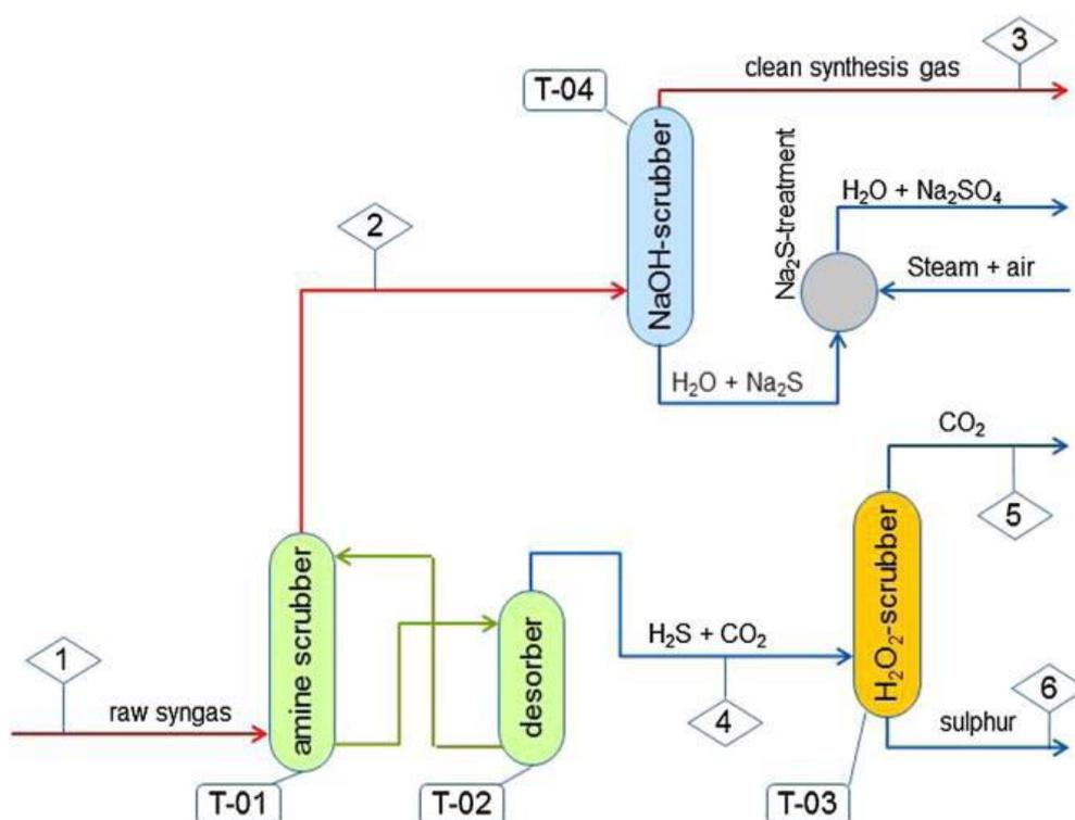
Figure 9: Block flow diagram of innovative gas cleaning concept
