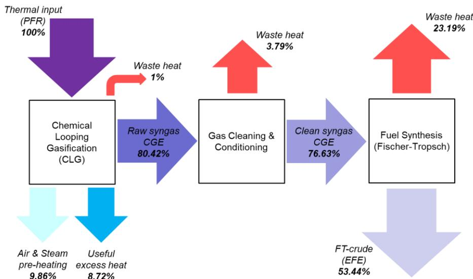
Figure 4: Heat balance for the entire BtL process chain for the model feedstock PFR.
