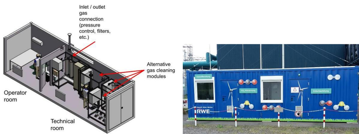
**Figure 10: 3D view and photo of mobile small-scale gas washing test rig**
