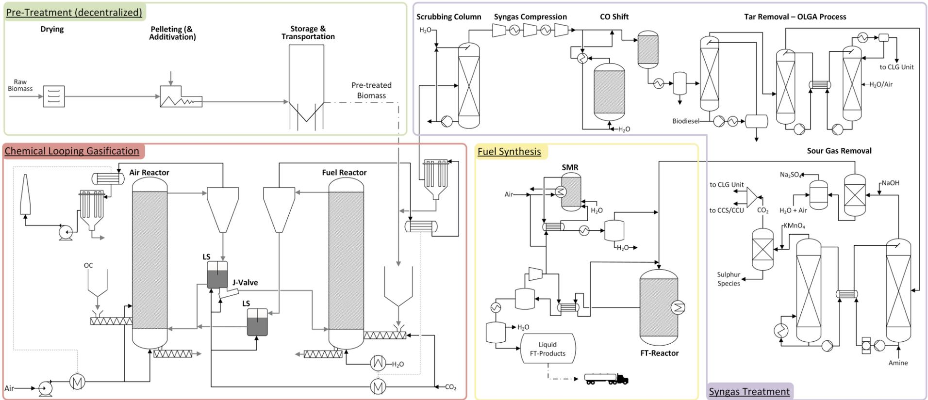
Figure 3: Simplified version of the process flow diagram for the CLARA biomass-to-liquid process chain.
