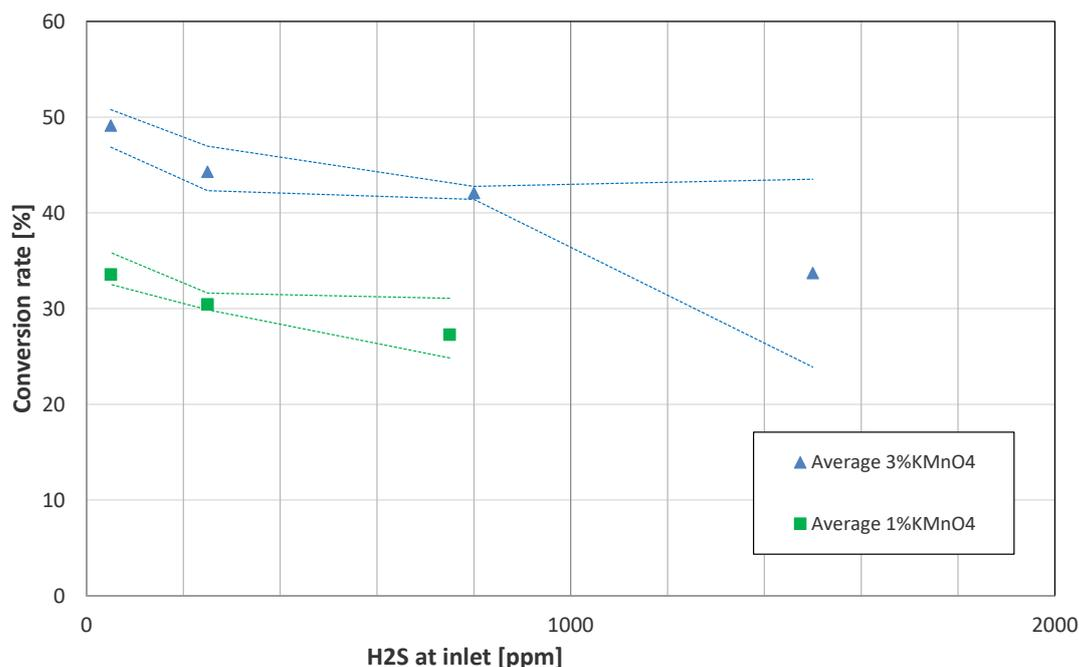
**Figure 11: Conversion of H<sub>2</sub>S to sulphur using KMnO<sub>4</sub>.**
