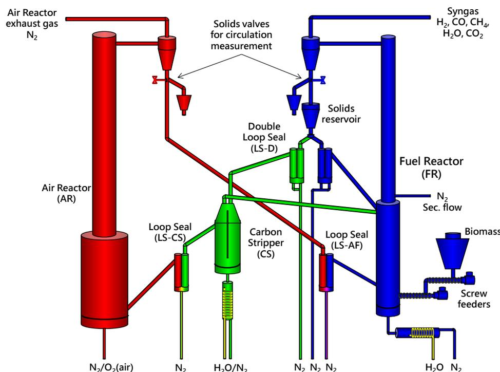
Figure 8: Layout of the CSIC facility (50 kW<sub>th</sub>) used for biomass fuelled CLG.
