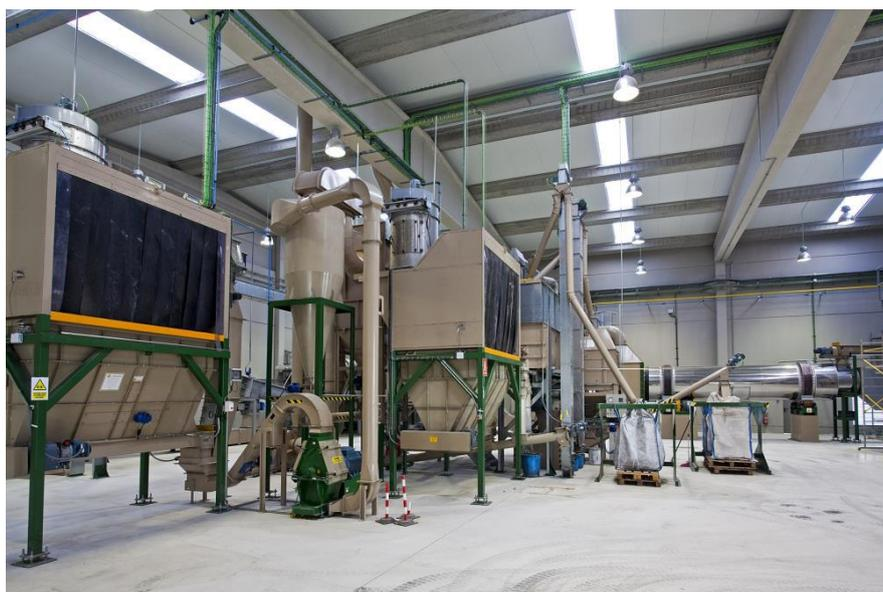
**Figure 7: Biomass pre-treatment unit at CENER facilities (BIO2)**
