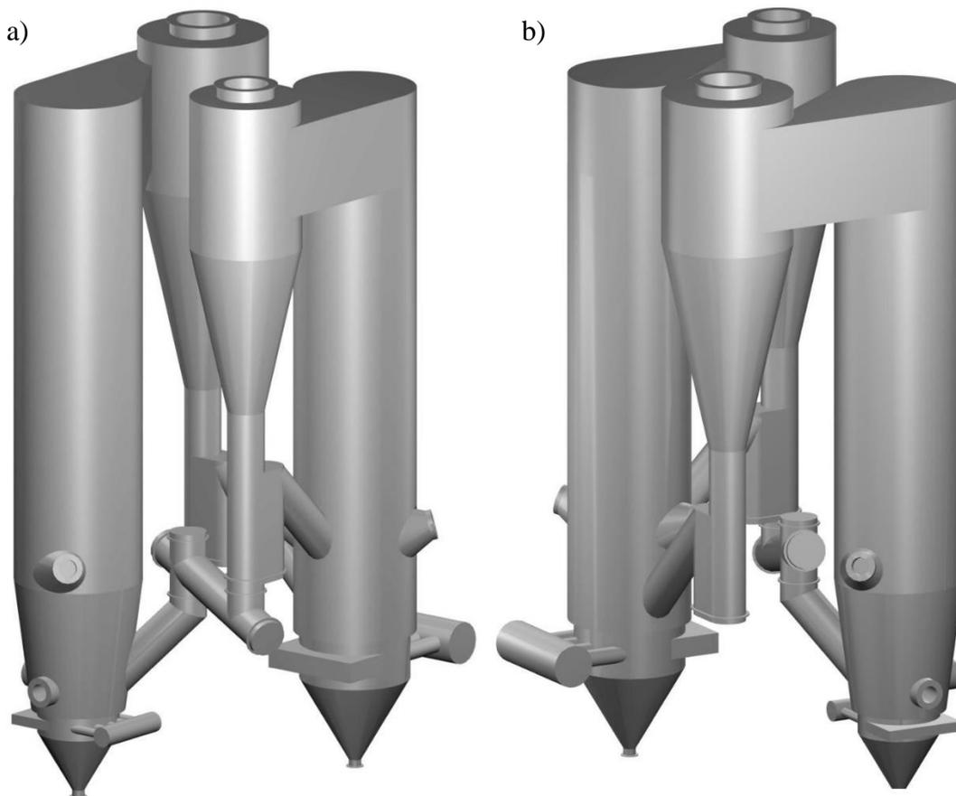
**Figure 6:** a) FR at left side, AR at right side; cyclone AR at front, cyclone FR in the back; J-Valve visible below the middle, b) FR at right side, AR at left side; cyclone FR at front, cyclone AR in the back.
