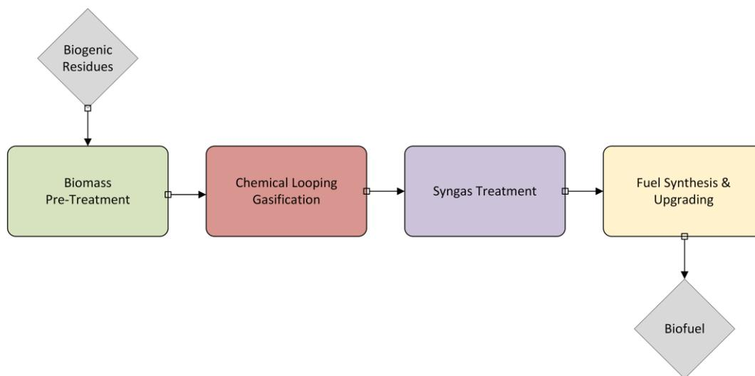
**Figure 1: Simplified scheme of full biomass-to-biofuel process chain.**
