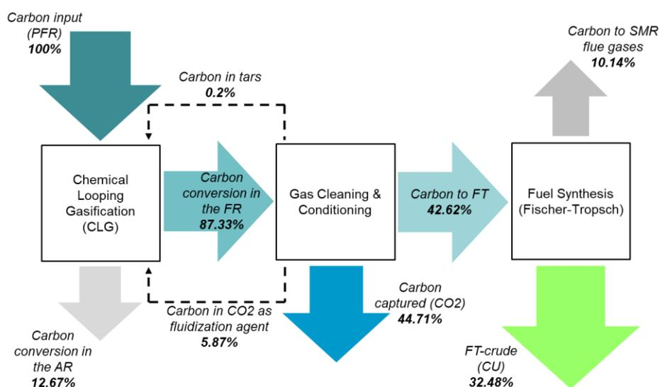
**Figure 5: Carbon balance for the entire BtL process chain for the model feedstock PFR.**
