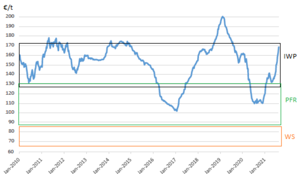
Figure 14 Evolution of historical industrial pellets (IWP) cost compared to calculated values for wheat straw pellet (WS) and pine forest residue pellets (PFR). Modified from [16]
