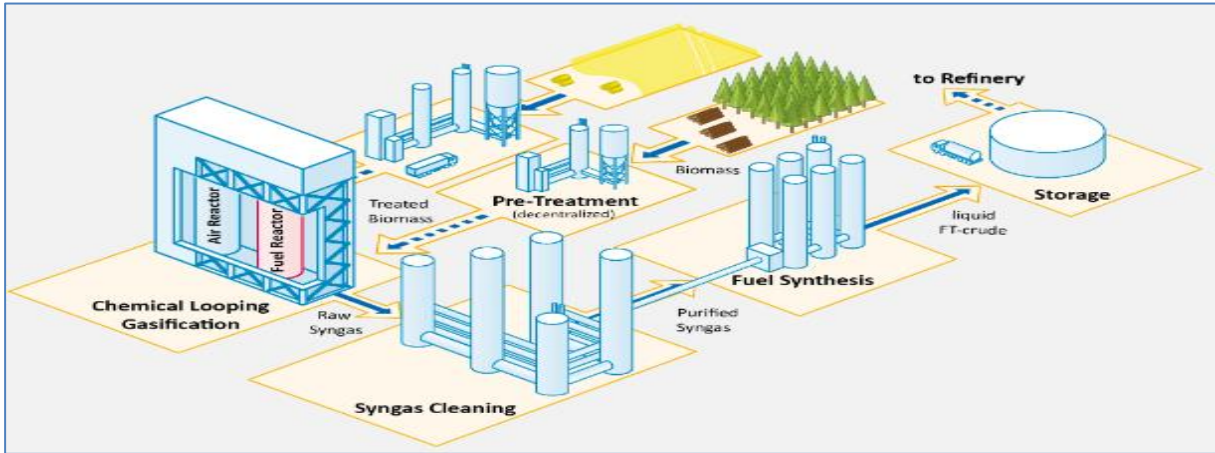
Figure 1. Schematic overview of the biomass-to-liquid process chain investigated in the CLARA project.
