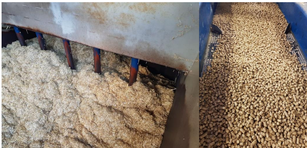
Figure 5: Straw pellet production. Left: fine grinded straw, left pelletized straw
