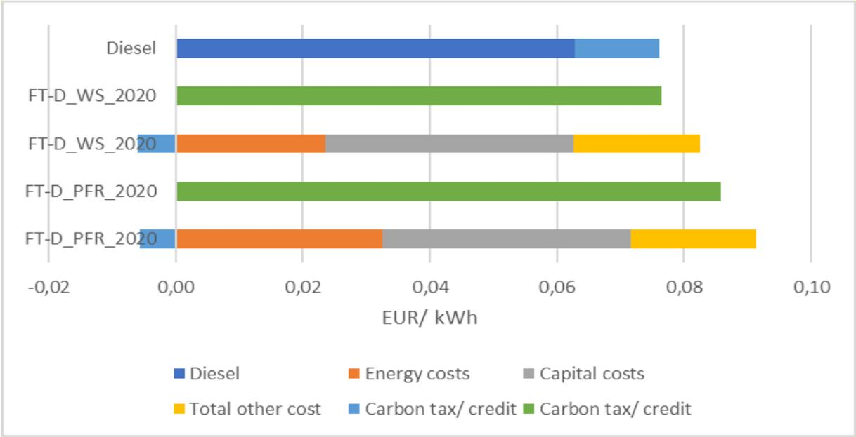
**Figure 3: Segmented total production costs for wheat straw-to-FT diesel & pine forest residues-to-FT diesel chains incl. CO<sub>2</sub> taxes for 2020 compared to corresponding Diesel price (€/kWh) for the EU<sup>4</sup>**
