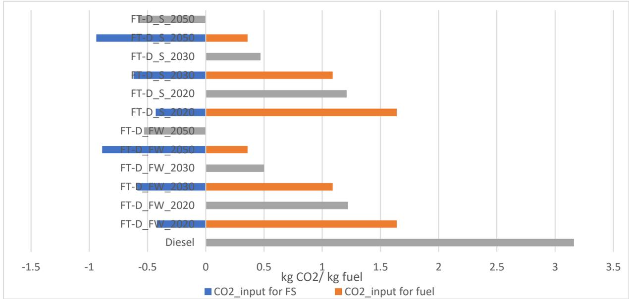
**Figure 5: CO<sub>2</sub> balances for forest wood-to-FT diesel & straw-to-FT diesel chains for 2020, 2030 and 2050 compared to corresponding Diesel CO<sub>2</sub> (TTW emissions) for the EU<sup>5</sup>**
