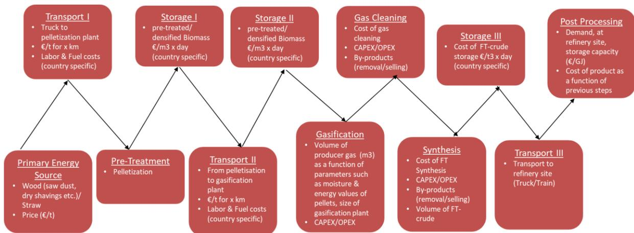
**Figure 1: Generic Biomass-to-Liquid fuel chain for CLARA process**
