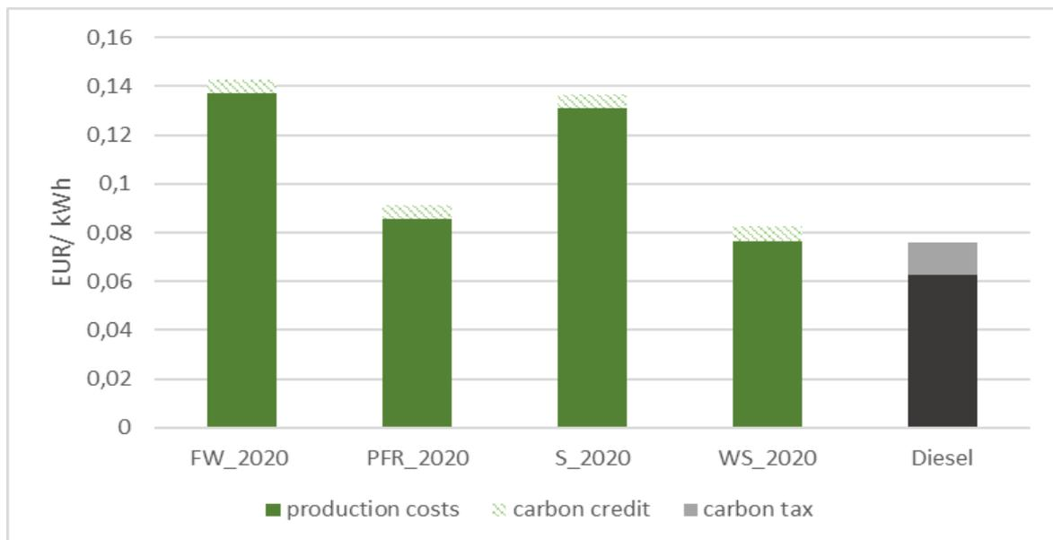
**Figure 8: Total production cost scenarios for forest wood-to-FT diesel, pine forest residue-to-FT diesel, straw-to-FT diesel and wheat straw-to-FT diesel chains incl. CO<sub>2</sub> taxes for 2020 (based on literature & data from CLARA project) compared to corresponding Diesel prices (EUR/kWh) for EU<sup>6</sup>**
